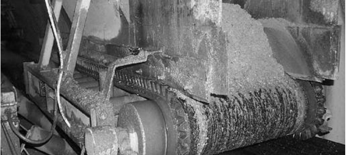
Sea-dredged aggregates working in wet, salty and aggressive environment! IP66/67 sealing – a MUST – often with re-greasable seals!
