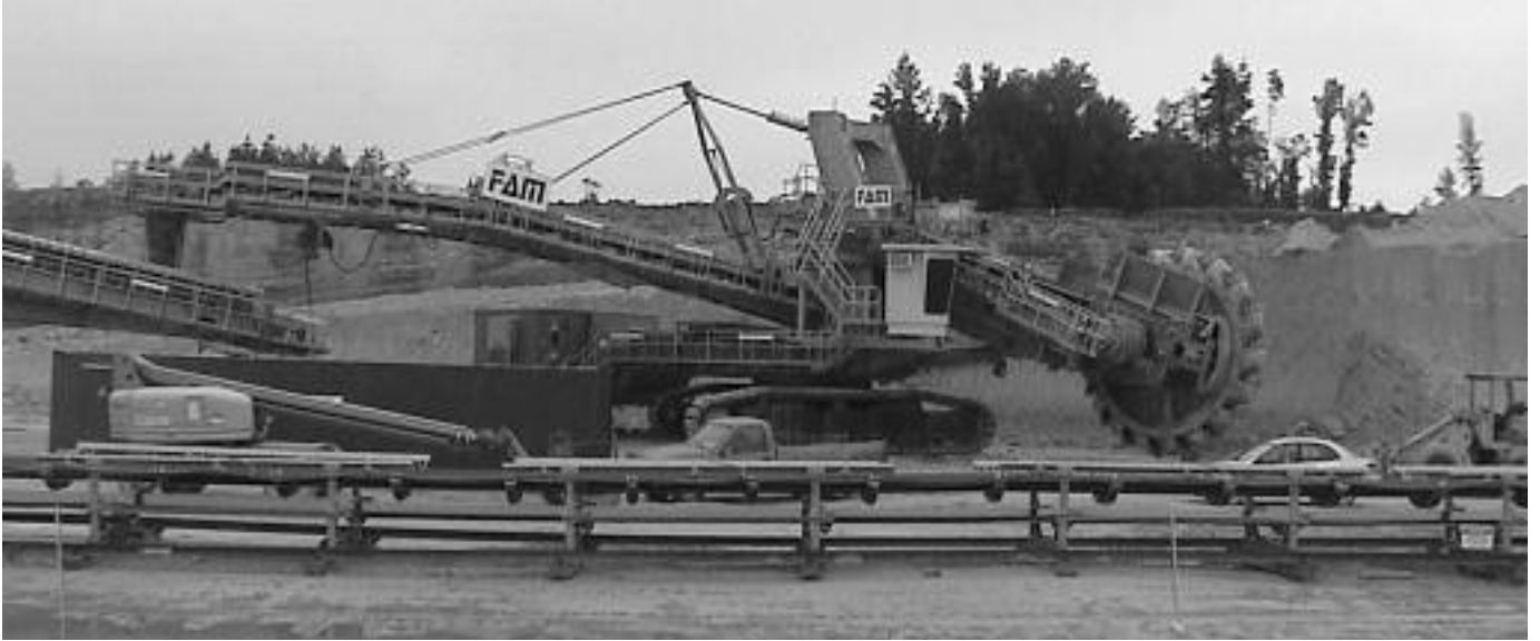
Excavator in a US cement application. Two Motorized Pulleys type 800H drive both the incoming & outgoing conveyors.
