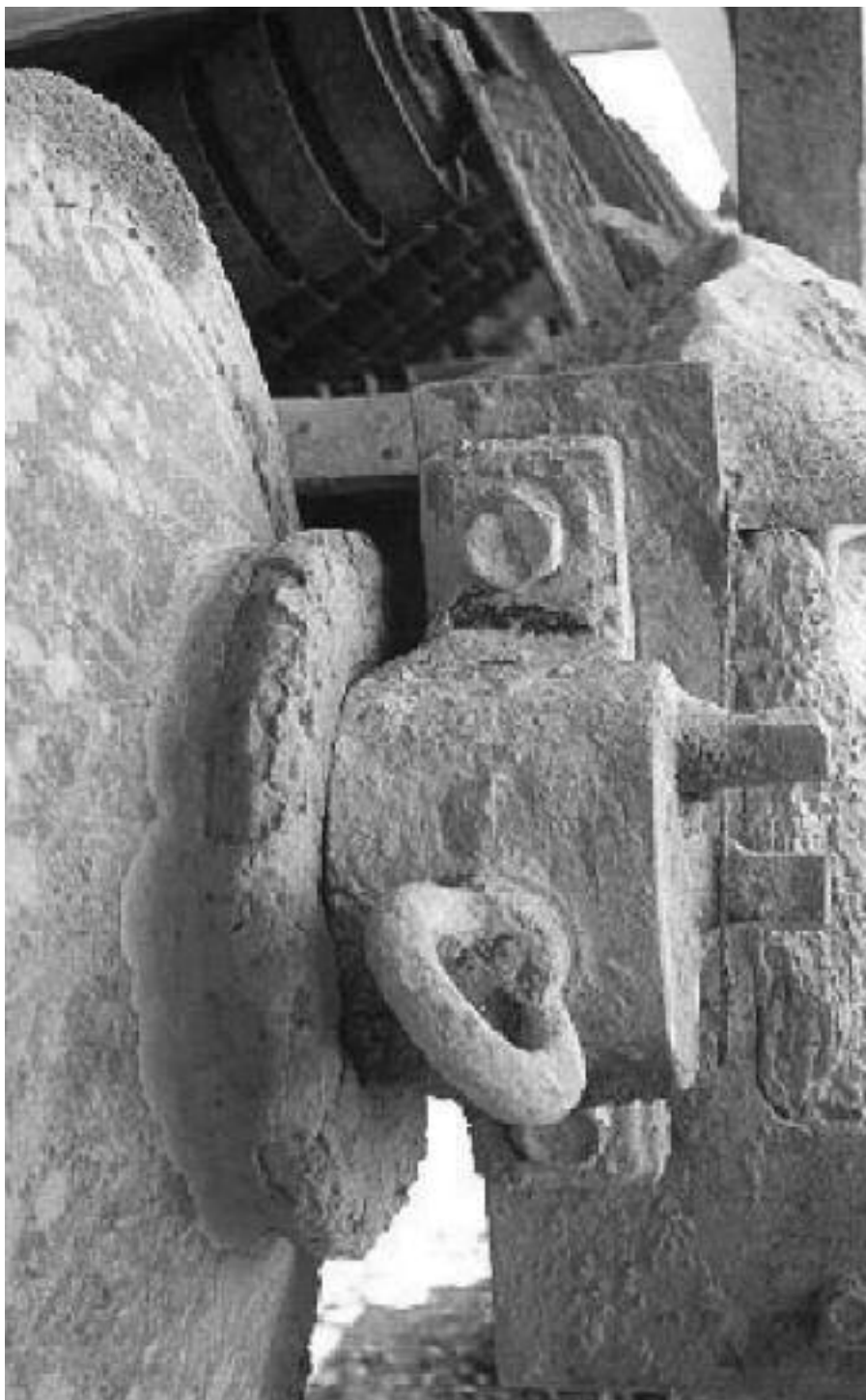
Application: Fertilizer and potash. Still in work after more than 30 years in an aggressive environment.
