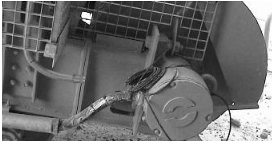
Excavator in a US cement application. Two Motorized Pulleys type 800H drive both the incoming & outgoing conveyors.
